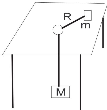
FIG. 3. The mass  $m$  is going around in a circle of radius  $R$  on a table. It is connected by a massless rope to  $M$ , hanging under the table.
