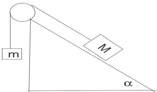
FIG. 4. The coefficient of static (kinetic) friction between  $M$  and plane is  $\mu_s$  ( $\mu_k$ ).
