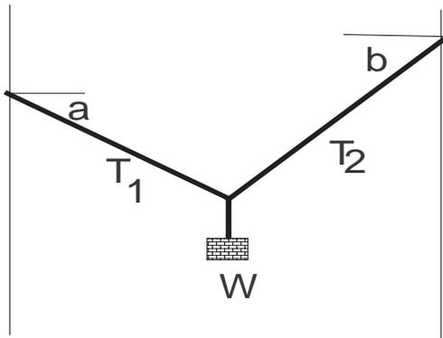
FIG. 1. Two strings making angles  $a$  and  $b$  meet at a point and support a mass  $10\text{ kg}$ .
